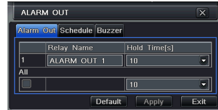
Fig 4-28 system configuration-alarm out
